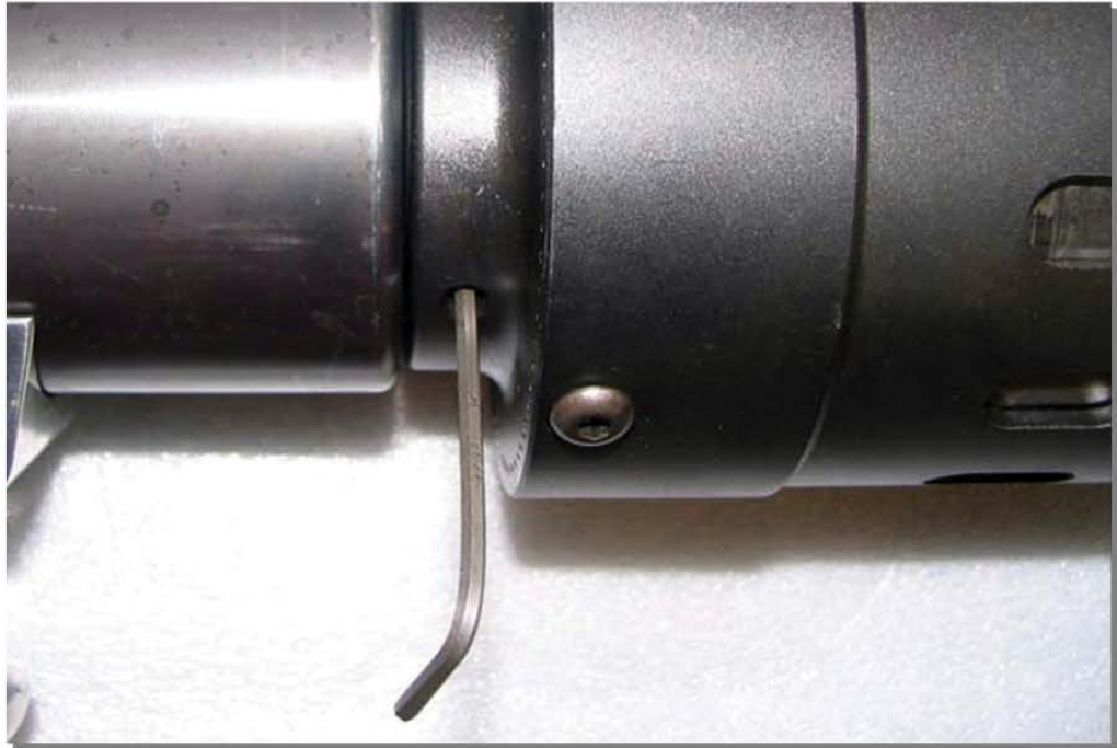
Figure 25. Tightening HYTORC Washer Set Screw
