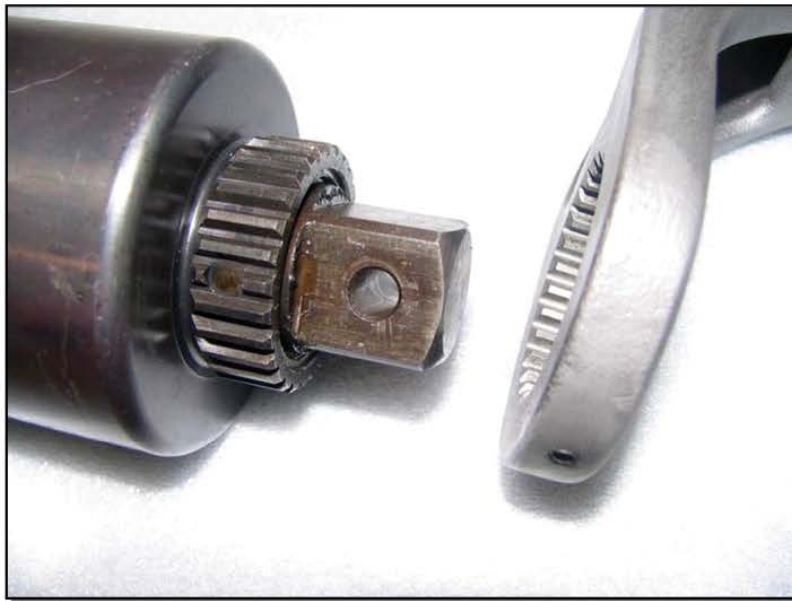
Figure 3. Installing a Reaction Arm
