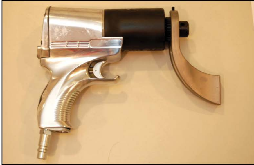
Figure 4. Reaction Arm installed
