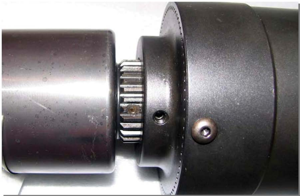
Figure 24. Aligning HYTORC Washer Socket Set Screw with Machined Recess in jGun Splines
