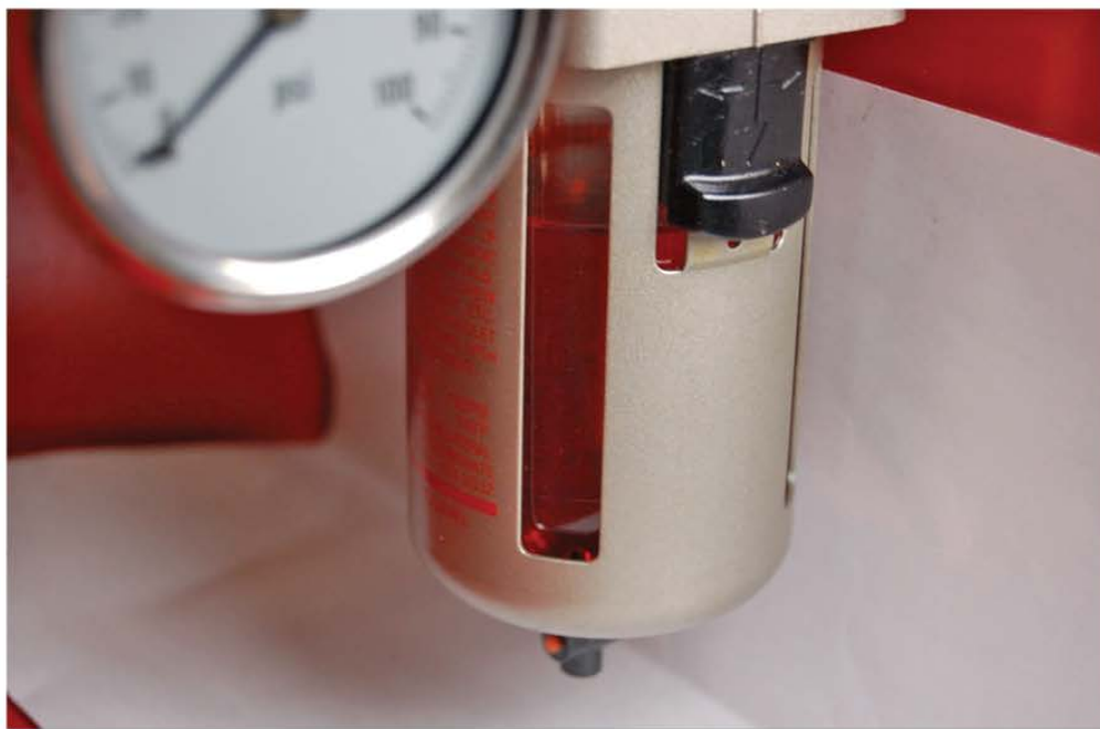
Figure 17. FRL Unit – Lubricator 2/3 Full of Oil
