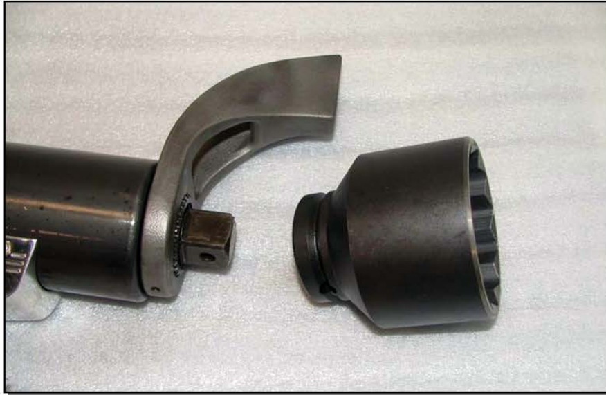
Figure 6. Installing jGun Socket
