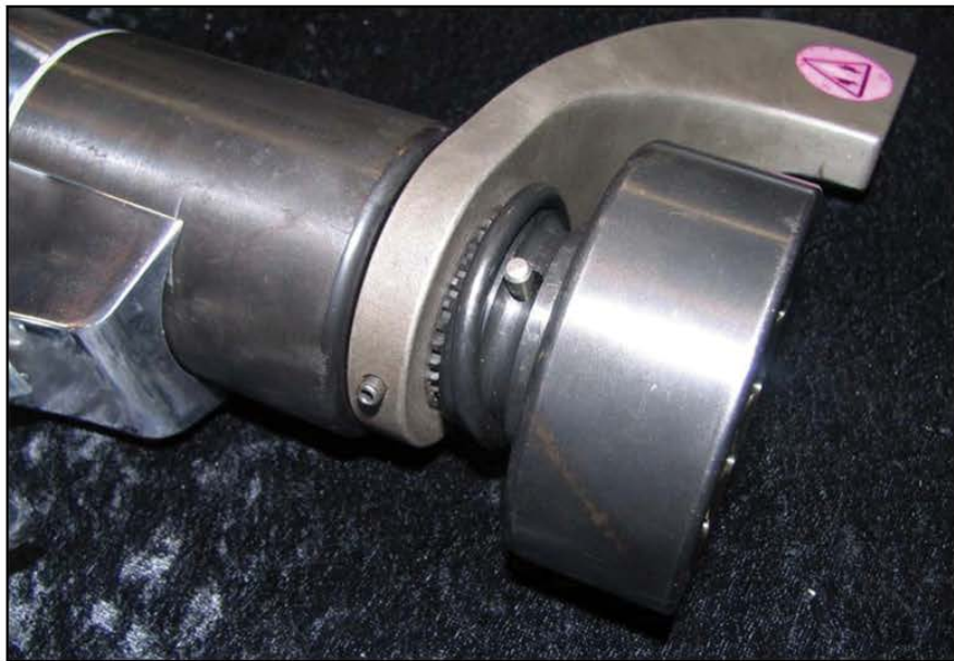
Figure 7. Installing Socket Locking Pin and Retaining Ring
