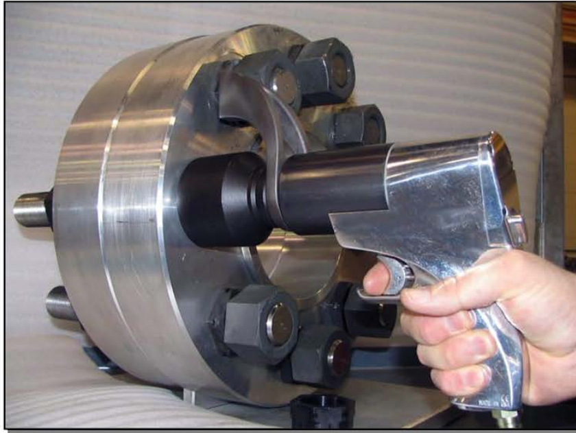
Figure 11. Using the jGun with a HYTORC Washer
