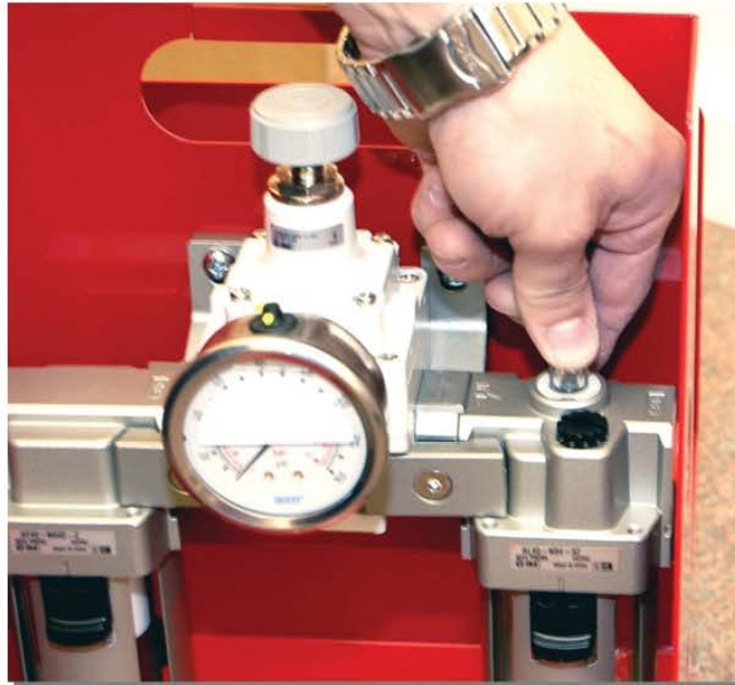
Figure 19. Adjusting FRL Oil Flow
