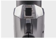
With a simple switch, the LITHIUM SERIES goes from high speed rundown mode to accurate final torque mode, eliminating the need for multiple systems on a job. The precision machined gearbox provides constant power without the vibration and noise found in impact guns. Adjust the power through the digital readout on the back of the gun to finetune the torque output for any job.
